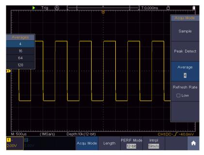
Figure 8-5 Reduce Noise level by using Average function
