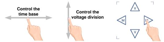
In the full screen, pinch and spread horizontally to change the time base; pinch and spread vertically to change the voltage division of the selected channel.
