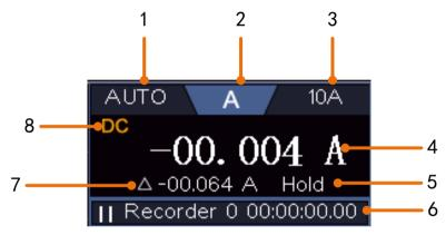
Figure 5-3 Multimeter Information Window
