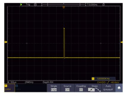
Figure 8-3 Capturing a Single Signal
