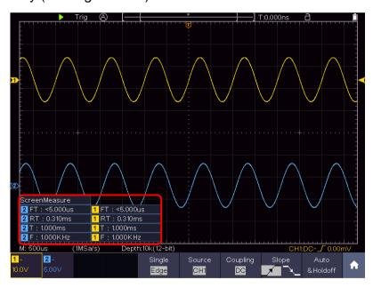
Figure 4-18 Automatic measurement
