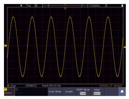
Figure 4-4 Sine(x)/x interpolation
