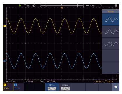
Figure 4-23 Autoscale Horizontal-Vertical multi-period waveforms
