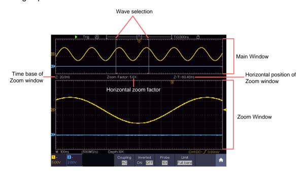
Figure 4-2 Waveform Horizontal Zooming Mode
