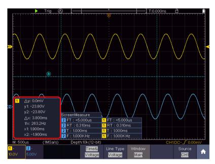
Figure 4-21 Time&Voltage Cursor Measurement
