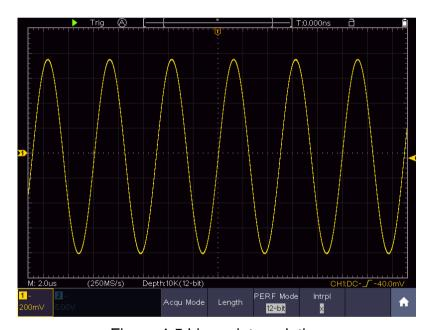
Figure 4-5 Linear interpolation
