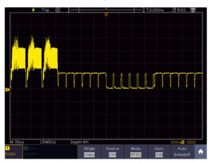
Figure 8-7 Waveform Captured from Video Field Trigger
