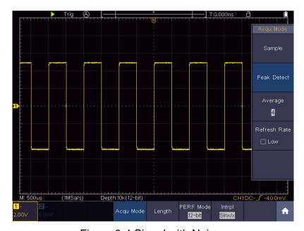
Figure 8-4 Signal with Noises
