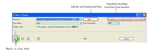
Figure 4-17: Play back waveform by software
