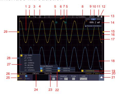
Figure 3-4 Illustrative Drawing of Display Interfaces
